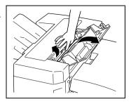
12 While holding misfeed clearing guide FN3 open, remove any paper.
